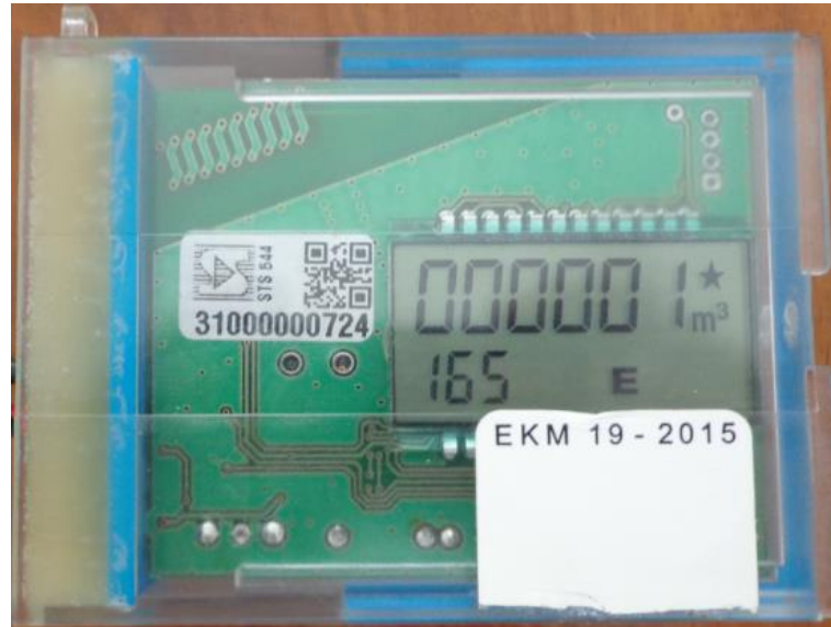
Illustration 1 Photograph of the prepaid water controller “PWC”
