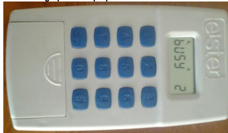
Illustration 2 Photograph showing the Customer Interface Unit (CIU)
